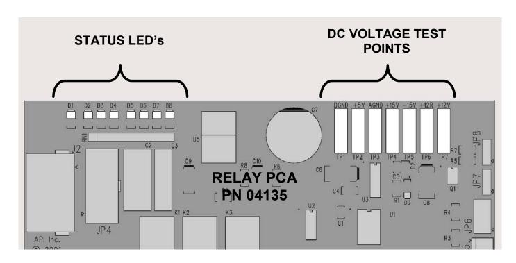
Figure 12-5: Relay Board Status LEDs
